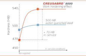
In addition, the super ductility of the retained austenite contributes to improve the lifetime in service by allowing larger micro shearing and thus delays the ultimate tearing of metal particles from the surface of the material exposed to the abrasive.
