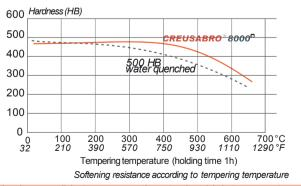
It is also possible to process the steel at high temperature  $500-550^{\circ}C$  ( $930-1020^{\circ}F$ ) (hot forming : bending, rolling) followed by a slow air cooling without inducing any significant drop of hardness (about 30-50 HB).
