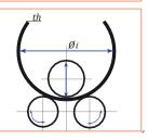
Creusabro®8000 <sup>°</sup> can be *hot formed* at a temperature of 500-550°C (930-1020°F) without any further heat treatment. At this temperature, forming requires lower power (according the reduction of the yield strength YS0.2) than the expected value at room temperature.
