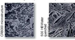
Such a microstructure differs from the rough acicular lamellar structure which is typical of the fully martensite steels (conventional 500 HB water quenched steels).
